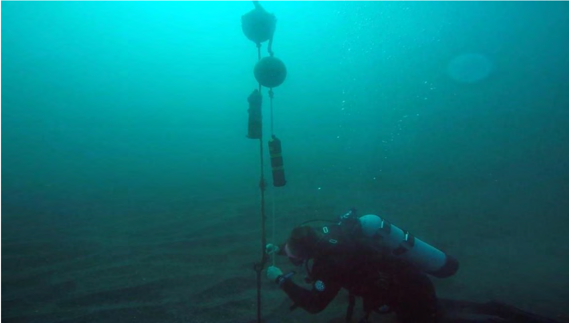
Figure 3.4. CINMS diver Ryan Freedman services a telemetry mooring anchored in soft sediment at Santa Barbara Island. Photo: Pike Spector/NOAA
